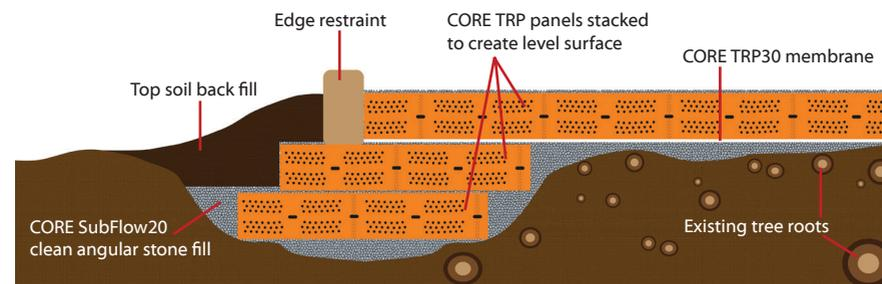
If the existing subsoil level within the RPA is sloping or has large undulations it may be necessary to stack the TRP panels to create a level surface for the final wearing course. Filling large dips and bumps with unstabilised fill material is not advised.
