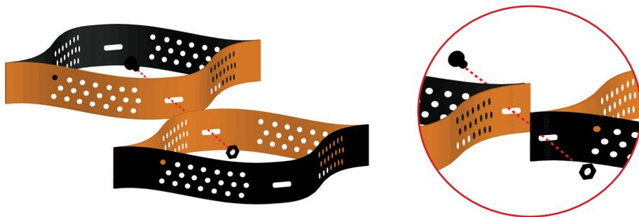
5. When connecting ends of adjacent panels align the elongated holes in the centre of the cell walls. Insert the stud through the holes in both panels and attach the securing nut.
