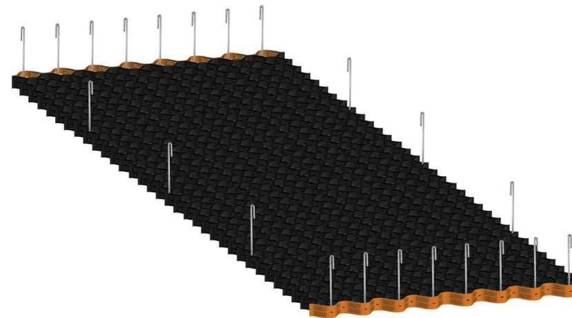
4a. Now measure 2710mm (the full width of the panel), and pin out the four corners to produce a fully expanded panel 2710 x 7380mm. Pin the remaining cells along each 2710mm end and evenly space 3 pins down each 7380mm side.
