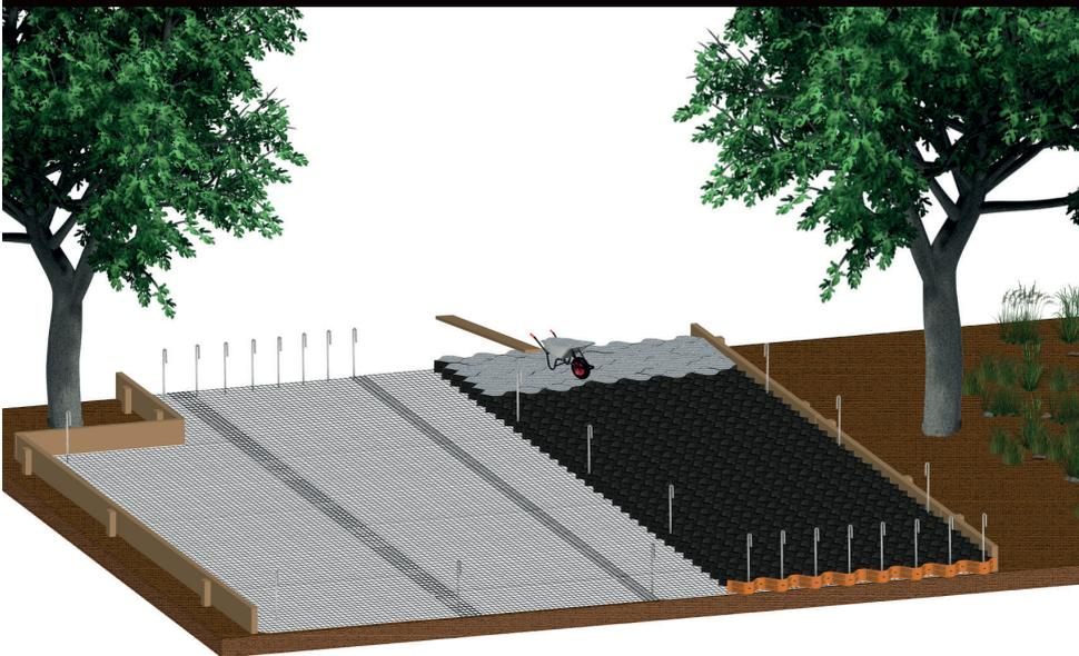
6. Starting at one end, begin to fill the cells progressively using CORE SubFlow20 or SubFlow40 clean angular 4/20 - 20/40mm cohesive stone. Limit the drop height to less than 1m to avoid collapsing unfilled cells.
