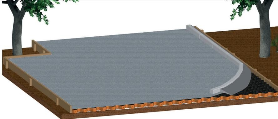
7. If the edging you installed in Step 2 is not the correct height or a different edging detail has been specified such as a granite sett or concrete kerb, this can be installed on top of the CORE TRP panel. The concrete haunching can go inside the cells of the TRP panel and on top to create an extremely strong and robust edge.
