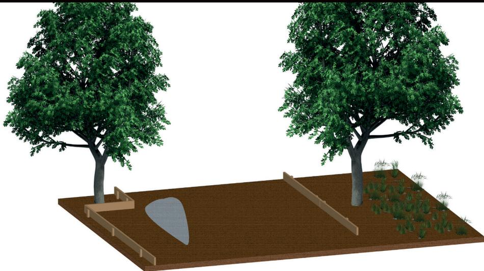
2. An edge restraint should be used around the perimeter of the TRP area. Tanalised timber and railway sleepers are the most commonly used edging for TRP systems. If a more substantial edging is required, concrete kerbs or path edgings can be used. *Edgings for the wearing course are explained in greater detail in Step 7.*
