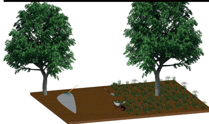
1. If agreed with the supervising arboriculturist remove the surface vegetation using hand held tools or herbicides. Cover any exposed tree roots using a suitable fill material. If large roots pretrude above ground the entire surface level may need to be adjusted. Please consult your supervising arboriculturist.
