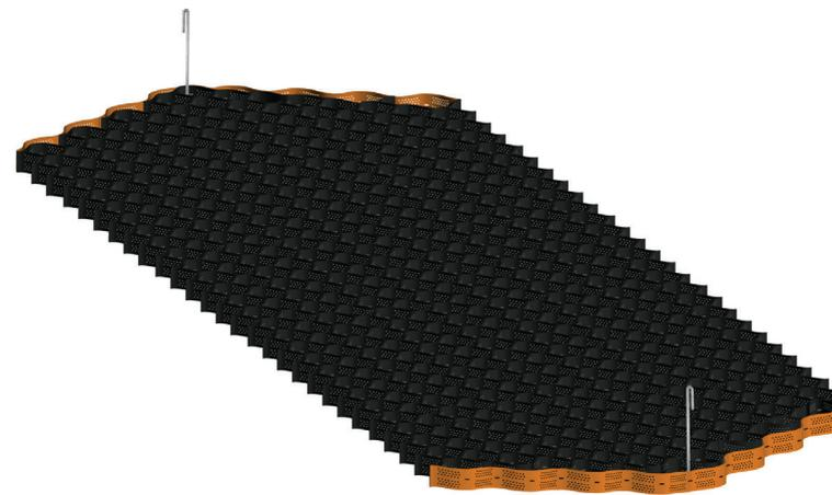
4. Measure in 1355mm from the edge restraint (half the width of the panel). Lay the collapsed CORE TRP panel and pin the centre cell closest to the end of the panel. Expand the panel to its full length (7380mm). Pin the centre cell at the opposite end.
